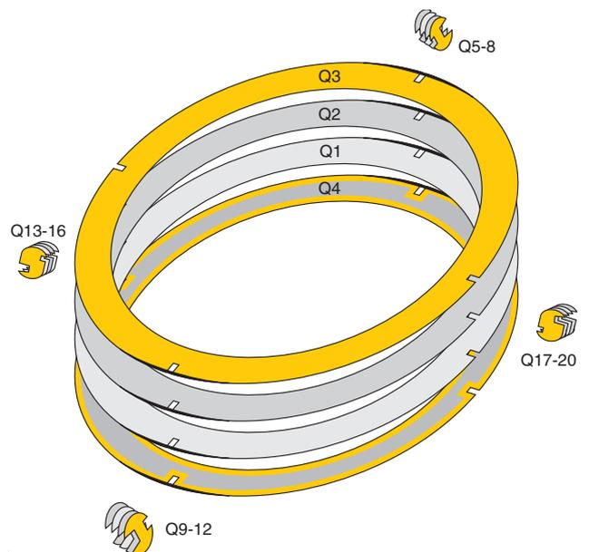
**Step 57:** With a pair of sharp scissors, cut off a narrow strip from the lunar orbit inner part 1 [Q1, sheet 11] at the two places denoted by black print. The ring, which is normally 14mm wide, is then only 13mm wide at these. The cut should be very gradual, so that you hardly notice the transition. *HINT:* the three other parts of the lunar orbit need to be cut as well, but only after they are glued in
