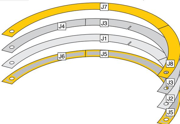
**Step 42:** Cut out the narrow slit depicted on the inner part, using a sharp knife. The slit is 1.3 mm wide and reaches to the centre of the ring. Use one of the metal pins to check the width: the pin should be a tight fit in the slit.
