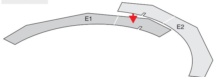
**Step 19:** Glue the horizon inner parts 1 and 2 [E1, sheet 5 + E2, sheet 6] together on their designated glue marks with their front sides facing each other. The edges as well as the rectangular cutout have to be exactly flush. The two parts only overlap on one third of their length, two thirds are protruding on each side.
